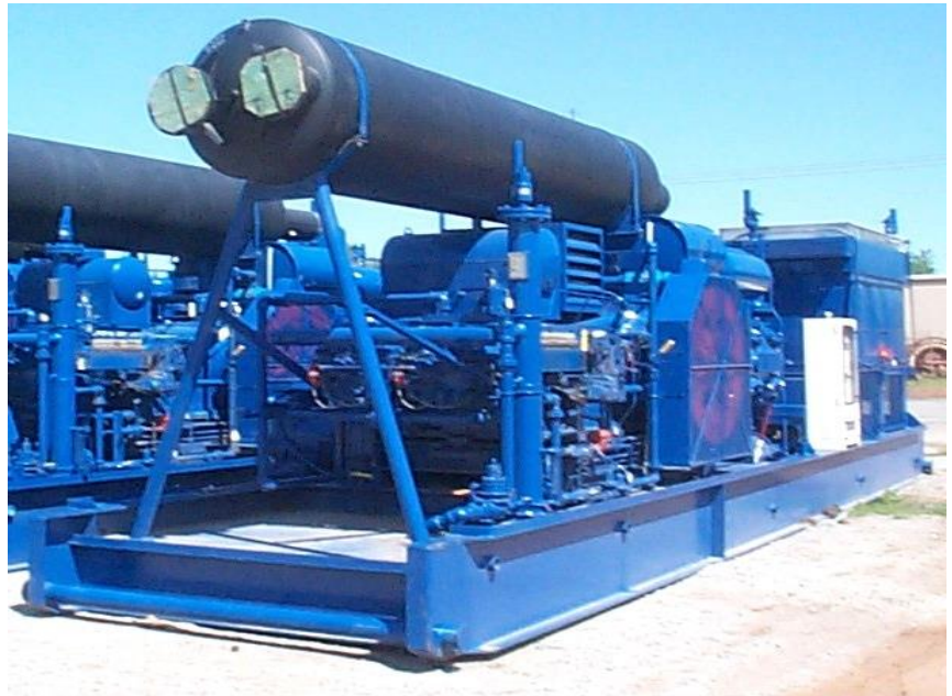
Figure 13: Narrow DPC-2802LE Package for Shipment on One Truck
